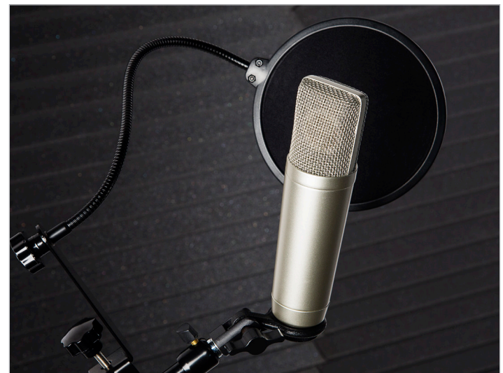
Fig. 4: A pop filter prevents wind noise and plosives from getting into a mic, and also blocks breath moisture, which can have negative effects on mic elements.
