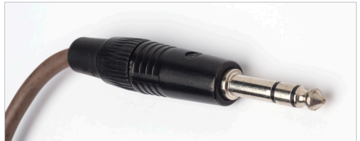
Fig. 6: A balanced (TRS) 1/4" phone plug. Note there are three sections, separated by black insulating bands—the tip, the ring, and the ground. These are also called stereo plugs when used to carry two independent left and right channel signals.
