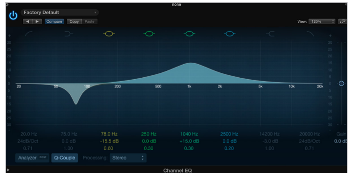
Fig. 22: Parametric filter response. A parametric filter can provide a peak or a notch in the frequency response.
