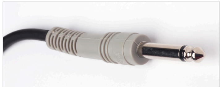
Fig. 5: An unbalanced 1/4" phone plug. Note the tip, the black insulating band, and ground. The flare toward the base of the jack provides a stronger grip when inserted into a jack.
