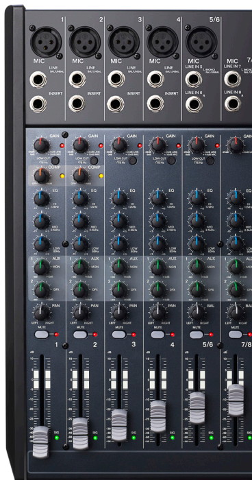
Fig. 17: Here's a typical channel strip. From top to bottom, there's an XLR input, a 1/4" line input for balanced or unbalanced lines (which you can use instead of the XLR in), TRS insert jack, mic/line switch to tailor the gain control characteristics to the chosen input, preamp gain control, three EQ controls for high/ mid/low frequencies, two aux send controls (one to a monitor out, one to the onboard digital effects), pan control, and level fader. Note the red clipping indicator to the upper right of the level fader, along with a yellow light to indicate when a channel is muted, as chosen by the Mute switch at the bottom of the channel strip.
