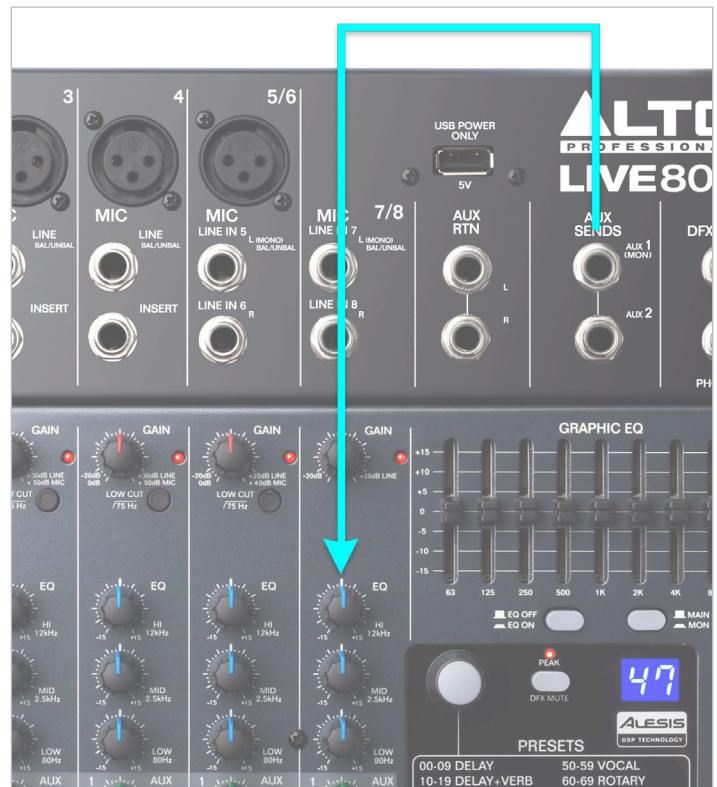
Fig. 20: The signals from several channels, for example multiple mics from a choir, go to Aux Send bus 1. Returning its output to a mixer input (in this case, the Line In 7/8 channel) lets you use the Line In 7/8 fader to alter the level of all mics together, without changing the balance of the individual mics.
