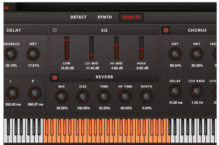
Fig. 23: A graphic EQ gets its name because the sliders draw a "graph" of the frequency response.
