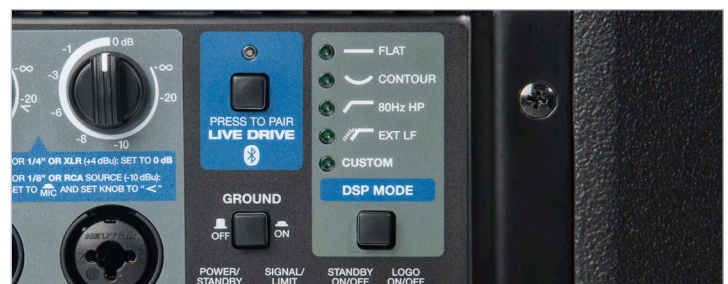
Fig. 26: The tone switch tailors the speaker's response to different environments.
