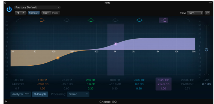
Fig. 21: Shelving filter response. There is a high-frequency boost, and low-frequency cut. The name “shelf” comes from the fact that after the response rises or falls, it levels off into a straight line.
