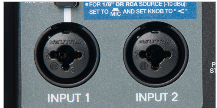
Fig. 10: The combination XLR jack is toward the left, and accepts both XLR and 1/4" phone plugs.
